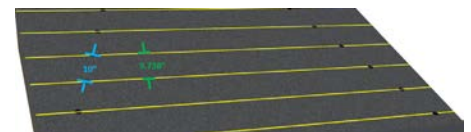
Figure E.7 Allowable (10-inches) vs Set (9.738-inches) exposure example.
