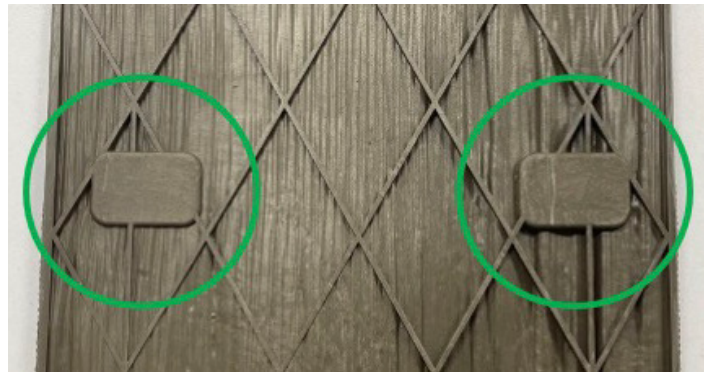
Figure 2.7.3 Fastener pads (back)
