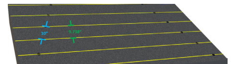
Figure E.6 Allowable (10-inches) vs Set (9.738-inches) exposure example.
