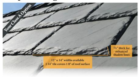
Bigger is better when it comes to EcoStar LLC's latest innovation. Empire Niagara Slate is a natural-looking, 5%" thick, synthetic slate roofing tile produced in 12" and/or 14" widths. This added size allows each Empire Niagara Slate 14" tile to cover one square foot of roof deck at the 10" exposure (100 tile/square), maintaining 2" headlap throughout. An additional 9" exposure option allows for the creation of unique looks using staggered, offset or random width installations.
